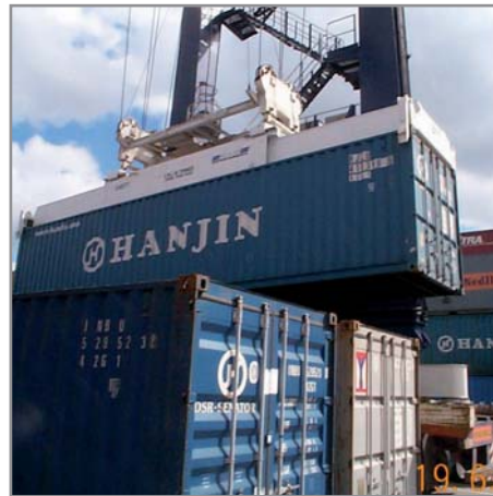
RAM 34/3500 All-electric telescopic spreaders.
